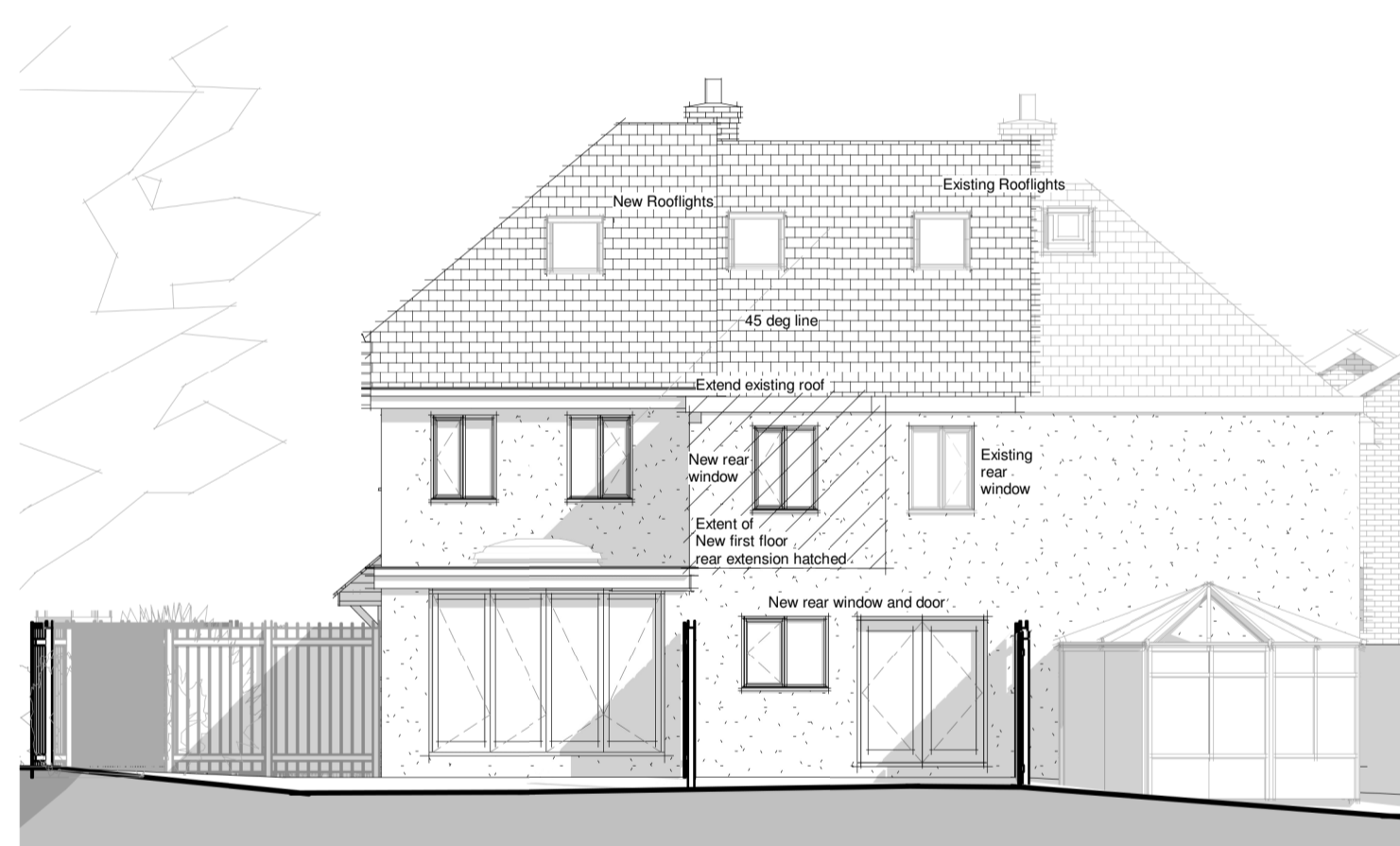
9 Terraced Rear Elevation 1 : 100
