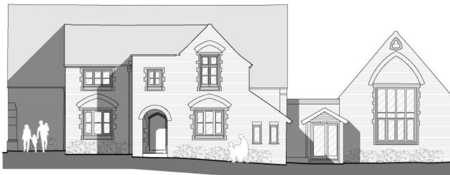
Fig. 3 – Proposed flank elevation illustrating the proposed two windows to match the existing windows and surrounds elsewhere on the building
