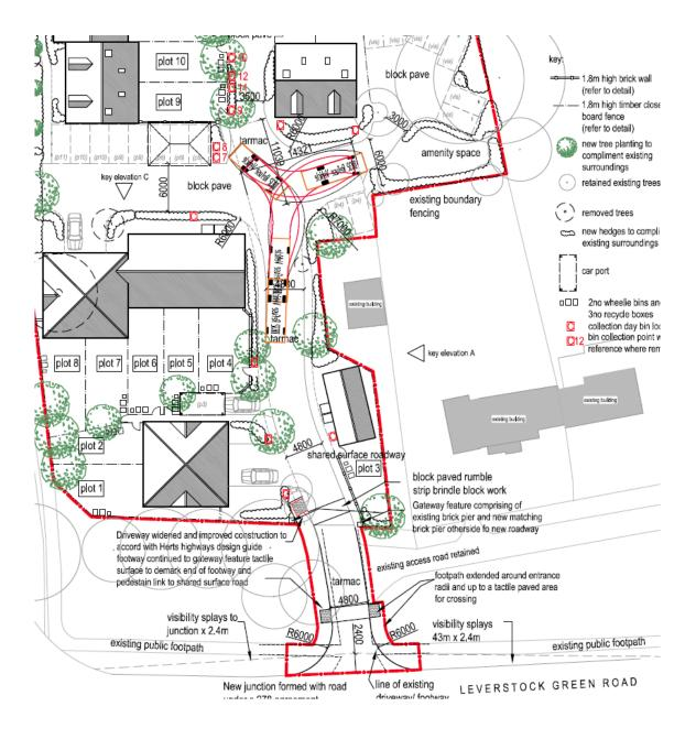
The internal estate road has a turning head dimensioned as indicated and is suitably sized to enable a refuse vehicle to turn as shown on the site layout and extract. In relation to the template- red lines represent the wheel tracking and the black lines the bodywork overhang of the vehicle.
